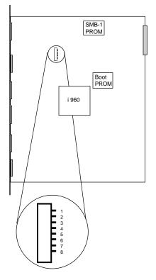
Figure 2-6. Location of Module DIP Switch
